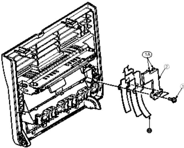
**Note:** Use care when replacing cable cover. Do not pinch, crimp, or cut cables or protective sheet.
