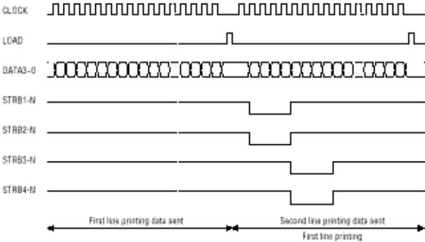
The printing operation is carried out in normal mode. Under ordinary circumstances such as when the power is turned on or when LOAD signal level is low, the normal mode is enabled.
