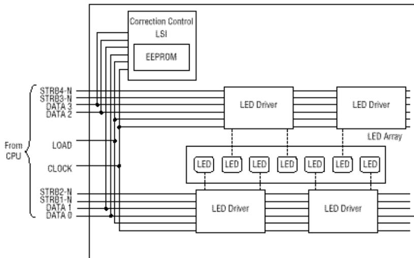
The LED correcting head is a 600 dpi head, with the LED drivers located on both sides of the LED array with a 300 dpi pitch spacing. The printing and correction data obtained from the CPU through four signal lines are sent to the LED array.
