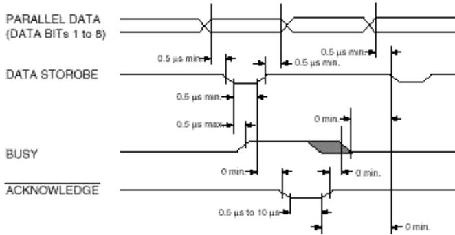
b) On-line ---> off-line switching timing by ON-LINE SW
