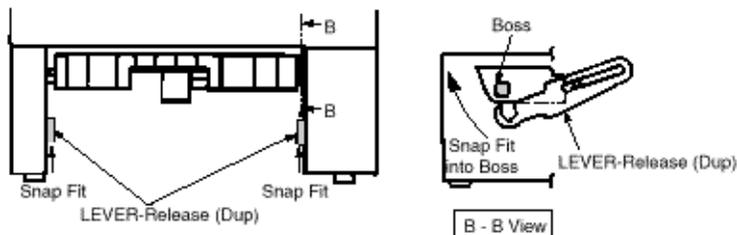
(4) After installing Duplex Unit, put back the Paper Cassette into 1st Tray.
