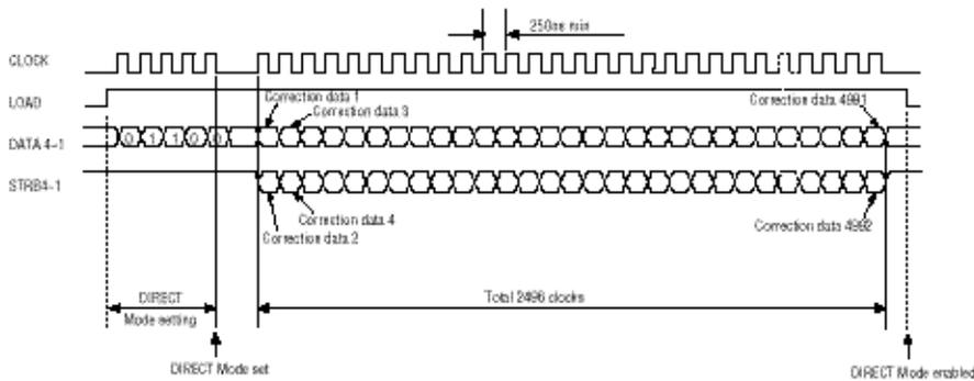
The LED driver corrects the LED illumination by controlling the LED current. The LED illumination can be set in 16 steps, with 7 steps in the direction of illumination increase in relation to the standard value, and 8 steps in the direction of decrease. For this reason, the LED correction data is a 4-bit data for each dot.
