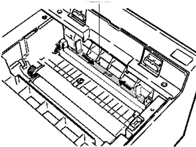
(3) Take the remove paper powder out of the printer unit in such a way as not to spill it, and then waste it.
