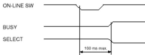
c) Off-line ---> on-line switching timing by ON-LINE SW
