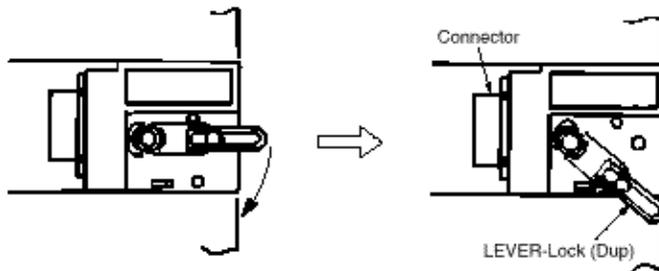
(3) From front side of printer, snap fit LEVER-Release (Dup) into the boss in Hopping Frame.
