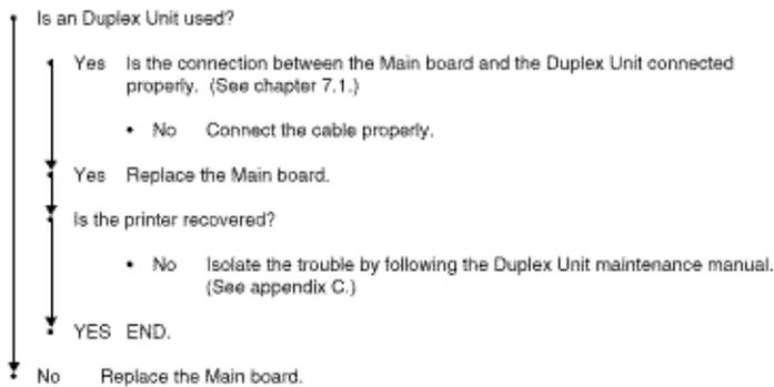
⑦ I/F time-out occurs between the printer and the operator panel (ERROR 80) .
