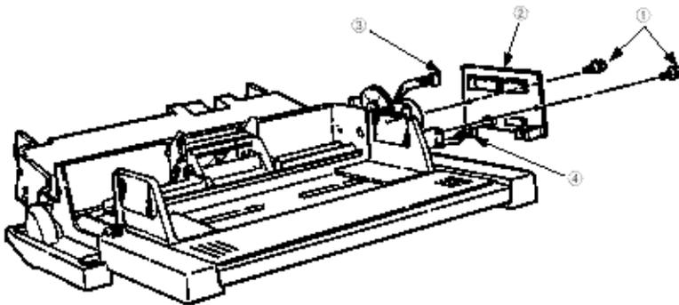
**Caution:** Be careful to set the sensor plate properly when mounting AOLE-PCB.
