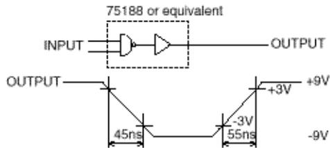
**Note:** The above signal level is for the case where 3KW x 15pF is being connected to the terminal.
