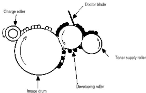
(2) The toner attracted to the developing roller is scraped off by the doctor blade, forming a thin coat of toner on the developing roller surface.
