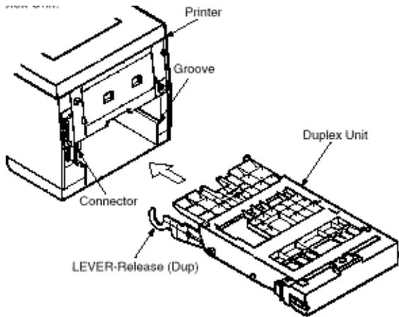
Printer and Duplex Unit will connect automatically with built-in connector.
