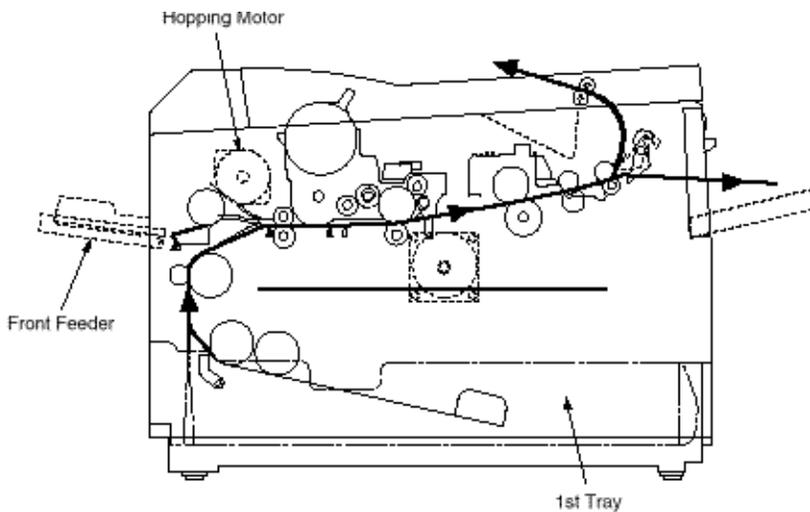
Turning the Hopping motor in direction a (CW) drives the 1st Hopping Roller. Turning the Hopping motor in direction b (CCW) drives the Front Hopping Roller. Gear C and Hopping roller build-in one-way bearing, so that turning each of these gears in reverse direction will not be transmitted to the corresponding roller.
