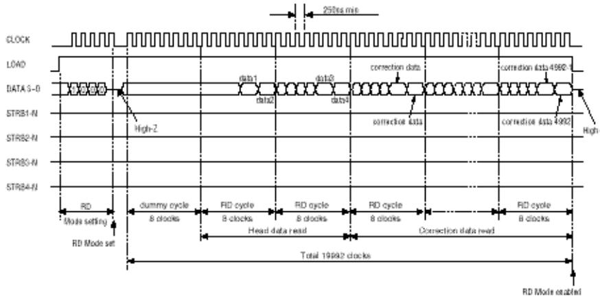
(2) Transfer of correction data to head driver correction data
