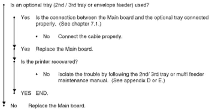
⑥ I/F time-out between printer and Duplex Unit (ERROR 83)
